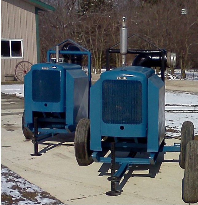
2 - 8 in. Gorman Rupp 88A2 Trash Pumps Powered by Ford F300 Gas 6 Cylinder Motors
